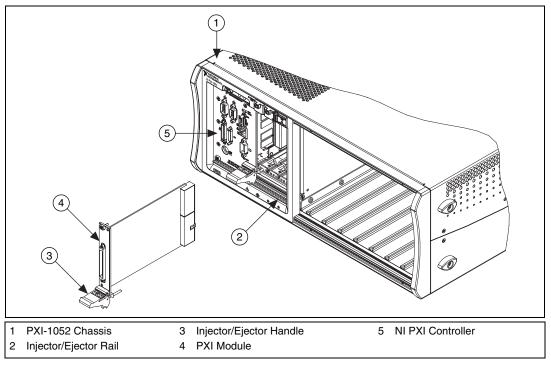
Figure 2-4. Installing PXI or CompactPCI Modules
